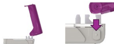
Figure B. To either remove or replace the cover, rotate it so that the opening points down. The cover can then be lifted or reattached by sliding along the flats until snapping into place. Once in place, it can easily be rotated closed or open.
